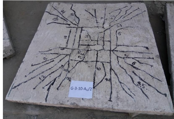
Fig.19: Cracking pattern of specimen (G-3-10-Ag/2).
